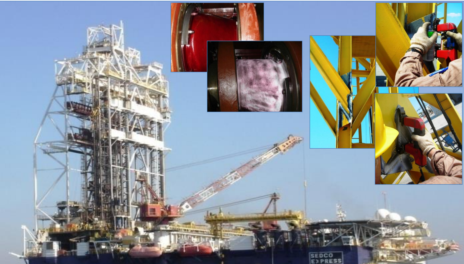
Pictures from visit to Offshore Drilling Platform for carrying out NDT / Non Destructive Testing (Liquid Penetrant Inspection – Magnetic Particle Inspection)
